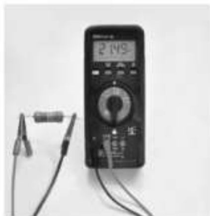
Fig 10.1 Resistance Measurement using Digital multimeter
